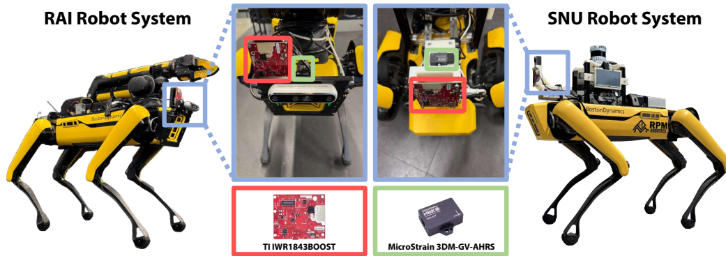
Figure 7. SNU and RAI sensor system deployment. Both systems include the same TI-mmWave radar, Microstrain IMU, and Boston Dynamics Spot quadrupedal robot, but are attached with different extrinsics.
